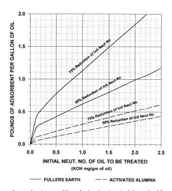
Approximate quantities of adsorbent material required for desired reduction in neutralization number of oil when using batch method of reclamation.
